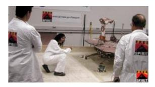
Mars Exploration Rover team members on July 21, 2009, tested how altering the order in which individual wheels turn for steering affects how those turns dig the wheels deeper into soft soil. From left: Alfonso Herrera, Vandana Verma, Bruce Banerdt.
