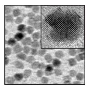
This is a high resolution electron micrograph image of magnesium oxide nanocrystals; the inset shows a single nanocrystal. Credit: Lawrence Berkeley National Laboratory
