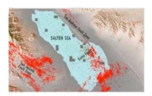
A seismic map of the Salton Sea area reveals the grid covered by the CHIRP instrument (green lines), faults (black lines) and bomb target sites (gray boxes). The red dots represent earthquakes that have taken place in the area since 1983. Credit: Scripps Institution of Oceanography, UC San Diego
