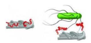
This graphic shows an aptamer attached to an electrode coated with single-walled carbon nanotubes interacts selectively with bacteria. The resulting electrochemical response is highly accurate and reproducible and starts at ultralow bacteria concentrations, providing a simple, selective method for pathogen detection. Credit: (C) Wiley-VCH 2009
