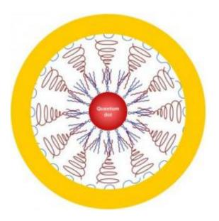
This is a quantum dot encapsulated in a gold shell. The total structure measures less than 20 nanometers across. Credit: University of Washington
