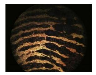
This is an optical microscope image of a fingerprint on brass. Credit: University of Leicester
