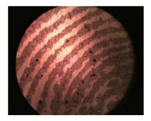
This is an optical microscope image of a fingerprint on brass. Credit: University of Leicester
