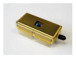
The CCD220 detector at the core of the OCam camera has 240 x 240 pixels and has a readout noise ten times smaller than detectors in current use, making it ideal for the faint light camera systems to be used on the second generation of Very Large Telescope instruments. It was developed by the British manufacturer e2v technologies. Credit: P. Balard/INSU-CNRS/ESO
