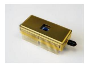
The CCD220 detector at the core of the OCam camera has 240 x 240 pixels and has a readout noise ten times smaller than detectors in current use, making it ideal for the faint light camera systems to be used on the second generation of Very Large Telescope instruments. It was developed by the British manufacturer e2v technologies. Credit: P. Balard/INSU-CNRS/ESO
