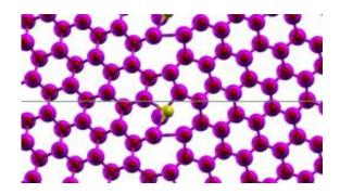
Irregularity in an ordered crystal structure. © Fraunhofer IWM
