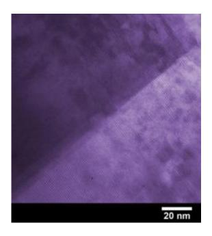
Electron microscope image of two superconducting thin films that meet at a six degree tilt boundary (the dark line running through the image). The numerous smaller lines that intersect the grain boundary at 90 degrees are the individual crystalline layers. The connection between the two films shows distortions in the superconducting layers, which severely limits current flow in these materials. Credit: F.J. Baca, US Air Force Research Lab
