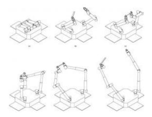
By connecting their endpoints, two reconfigurable robots autonomously change their configurations by altering the lengths of their arms and twisting their joints. Image credit: Aghili and Parsa. ©2009 IEEE.
