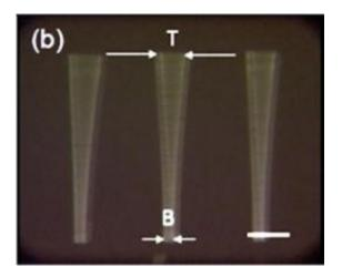
The artificial cilia are flexible rubber fingers less than 1/100 of an inch long, and 1/1000 of an inch wide. The tips shown here vibrate 65 times per second. Credit: University of Washington
