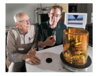
Sandia researchers Jack Houston (left) and Nathan Moore examine a tiny salt block while the screen behinds them shows the magnified tip of the Sandiadeveloped interfacial force microscope (device in the foreground) performing another materials interrogation. The device was developed by Houston. Credit: Sandia National Laboratories
