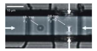
The integrated optical trap allows independent manipulation of trapped microbeads as shown in this view of two microbeads trapped by two different dual-beam traps. Image courtesy of H. Schmidt.
