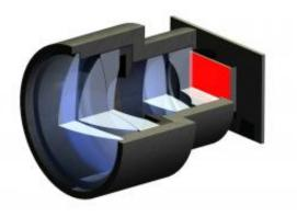
Model of the mini beamer: the OLED display can be seen to the right at the back. The lens system projects the image onto a wall. © Fraunhofer IOF
