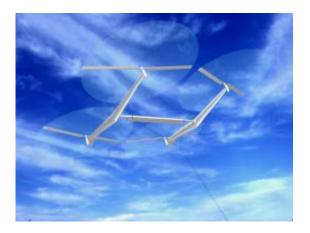
A Sky WindPower kite of turbines might capture wind energy with spinning rotors and send electricity to the ground through the wire that tethers it. (Ben Shepard)
