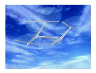
A Sky WindPower kite of turbines might capture wind energy with spinning rotors and send electricity to the ground through the wire that tethers it. (Ben Shepard)
