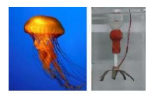
(Left) A living jellyfish and (right) a jellyfish robot made of electro-active polymer artificial muscle. Both jellyfish move by contracting the bell to generate a pulsating motion. Image: Yeom and Oh.
