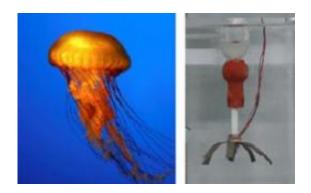
(Left) A living jellyfish and (right) a jellyfish robot made of electro-active polymer artificial muscle. Both jellyfish move by contracting the bell to generate a pulsating motion. Image: Yeom and Oh.
