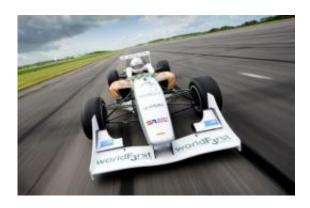
The WorldFirst Formula 3 racing car drives down the straight of a test track at Bruntingthorpe near Lutterworth, in Leicestershire. The steering wheel is made from a polymer derived from carrots and other root vegetables while the seat is flax fibre shell, soy bean oil foam and recycled polyester fabric.
