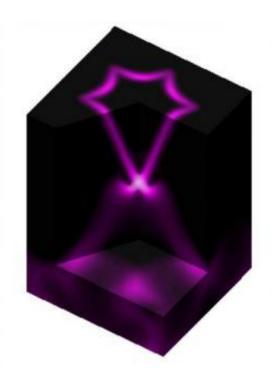
This is a surface electron band structure of bismuth telluride. Credit: Image courtesy of Yulin Chen and Z. X. Shen
