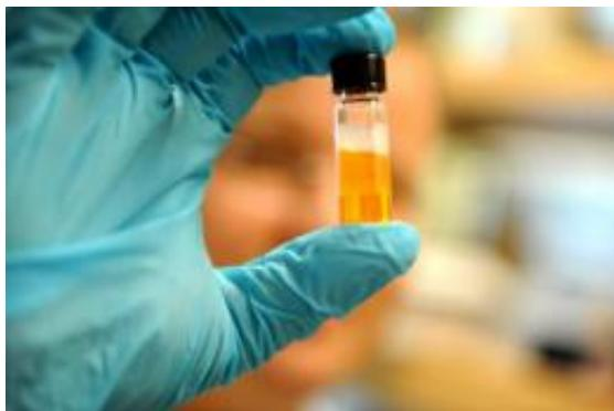
This is a vial of nanocrystals in solution, which serve as "electronic glue" for semiconductor-based technologies. Credit: Dan Dry
