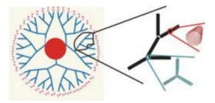
The figure illustrates a hierarchical network of carbon nanotubes mimicking a cell's protein network to connect a small heat source (red area) to a larger area that serves as a heat sink.
