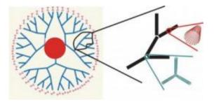
The figure illustrates a hierarchical network of carbon nanotubes mimicking a cell's protein network to connect a small heat source (red area) to a larger area that serves as a heat sink. Credit: Graphic / Markus Buehler, MIT
