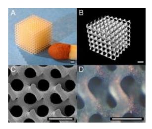
Biodegradable carrier structure made using stereolithography. The newly-developed polylactide-based resin makes it possible to replicate three-dimensional digital structures very accurately. The white bar is 500 micrometre in length. A) photograph of a porous structure fabricated using stereolithography. B) Micro-CT scan of the structure fabricated. C) Electron microscope image. D) Porous structure sown with bone cells.
