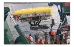
The hybrid remotely operated vehicle Nereus may be tethered or untethered to a mother ship. Credit: WHOI
