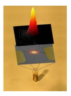
Artist's rendering of the two techniques used to "see" the carbon nanotube lamp: visible light microscopy (top) and electron microscopy (middle). The nanotube filament is 1.4 micrometers long but only 13 nanometers (about 100 carbon atoms) in diameter. Image: UCLA
