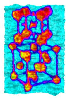
The arrangement between atoms of a film of strontium titanate and the single crystal of silicon on which it was made is shown on the left. When sufficiently thin, the strontium titanate can be strained to match the atom spacing of the underlying silicon and becomes ferroelectric. On the right, this schematic has been written into such a film utilizing the ability of a ferroelectric to store data in the form of a reorientable electric polarization. Credit: Jeremy Levy, University of Pittsburgh
