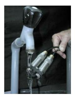
Placed in a stream of flowing water, a sensor head provides real-time quality analysis. Credit: AFTAU
