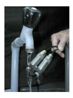
Placed in a stream of flowing water, a sensor head provides real-time quality analysis. Credit: AFTAU
