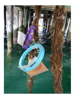
Sachets containing resin beads that absorb algal toxins are used to monitor toxins in coastal waters. Photo by Meiling Roddam, UCSC.
