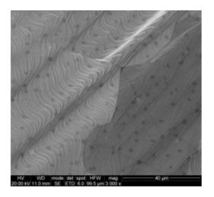
This is a scanning electron microscope image of copper foil fully covered with graphene. Credit: Xuesong Li and Weiwei Cai
