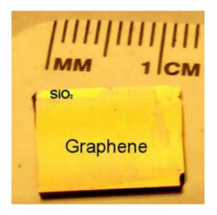
This is a one centimeter-by-one centimeter graphene film transferred to a silicon wafer with a silicon dioxide top layer. Credit: Xuesong Li and Weiwei Cai
