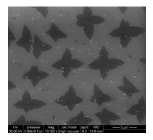
This is a scanning electron microscope image of graphene "seeds" on copper foil. Credit: Xuesong Li and Weiwei Cai
