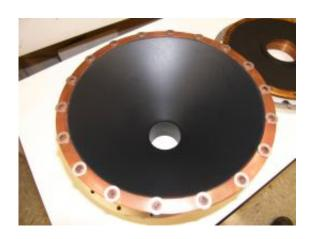
Carbon nanotubes (black coating in photo, right) form the inner lining of NIST's new laser power meter, enabling the copper instrument to withstand the intensity of military lasers while precisely measuring their power. Laser light is distributed evenly inside the water-cooled cavity by a mirror (diagonal component at center of graphic). Credit: C. Cromer/NIST
