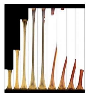
This shows progressive images of a mechanophore linked elastomer during tensile loading. After the polymer reaches a critical strain, a force-induced red color results from selective covalent bond cleavage in the mechanophore just prior to failure. Credit: Beckman Institute ITG, Darren Stevenson and Alex Jerez
