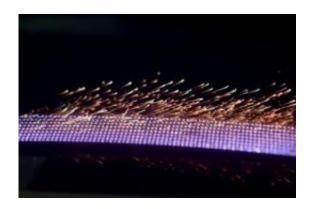
The laser beam is guided and focused by means of a process adapted manufacturing system. This allows thousands of holes to be burned into a silicon wafer in one second. Image: Fraunhofer ILT
