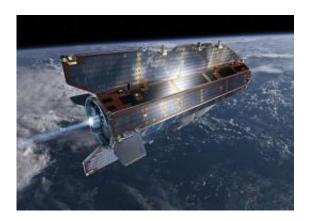
GOCE orbit is so low that it experiences drag from the outer edges of Earth's atmosphere. The satellite's streamline structure and use of electric propulsion system counteract atmospheric drag to ensure that the data are of true gravity. Credits: ESA - AOES Medialab
