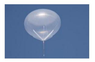
This picture shows the high-altitude balloon fully expanded to a diameter of 459 feet. The red immediately below the balloon is the parachute. The LEE payload of cosmic ray detectors is at the bottom of the chute shrouds. This photo was taken through a telescope by Drew Denney, NASA Columbia Scientific Balloon Facility.
