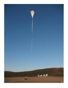
Launch of high-altitude balloon carrying cosmic ray detectors over Kiruna, Sweden, May 17, 2009. The balloon is made of a polyethylene film (the same material used to make trash bags) and weighs 4,150 pounds without its payload. Photo by James Roth/University of Delaware
