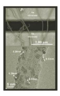
Hybrid sensor fabrication process: (top) SEM image of a few MWCNTs spanning across two neighboring Au fingers of the interdigitated electrode; (bottom) HRTEM image of a MWCNT uniformly coated with SnO nanocrystals.
