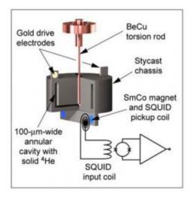
A torsion oscillator shakes a sample of frozen helium back and forth like a washing machine agitator, and gives experimenters information about the state of the matter inside. At temperatures near absolute zero some of the helium goes into a frictionless "supermatter" state and offers less resistance to being pushed back and forth. The entire apparatus is about the diameter of a quarter. Image: Davis Lab
