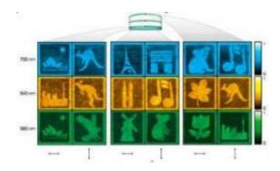
Recorded with multiple dimensions of light and layers, a 5D DVD could have a data capacity of 1.6 terabytes. Image credit: James Chon/Swinburne University of Technology.
