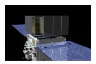
The Large Area Telescope (LAT) on Fermi detects gamma-rays by tracking the electrons positrons they produce after striking layers of tungsten. This ability also makes the LAT an excellent tool for exploring high-energy cosmic rays. Credit: NASA/Goddard Space Flight Center Conceptual Image Lab
