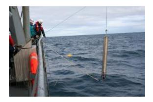
A photo of a hydrophone being deployed in the North Atlantic.
