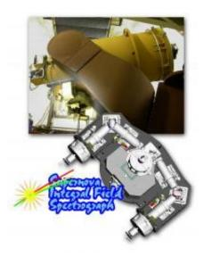
The SuperNova Integral Field Spectrograph (SNIFS) was designed and integrated by SNfactory collaborators based at the University Pierre and Marie Curie (UPMC) in Paris and the University of Lyon. Mounted on the University of Hawaii's 2.2-meter telescope on Mauna Kea, SNIFS integrates spectral and brightness information from numerous regions in compound images of each supernova and its host galaxy. Credit: Nearby Supernova Factory
