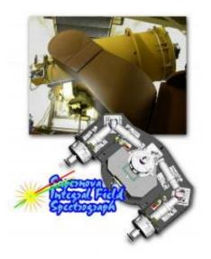
The SuperNova Integral Field Spectrograph (SNIFS) was designed and integrated by SNfactory collaborators based at the University Pierre and Marie Curie (UPMC) in Paris and the University of Lyon. Mounted on the University of Hawaii's 2.2-meter telescope on Mauna Kea, SNIFS integrates spectral and brightness information from numerous regions in compound images of each supernova and its host galaxy. Credit: Nearby Supernova Factory
