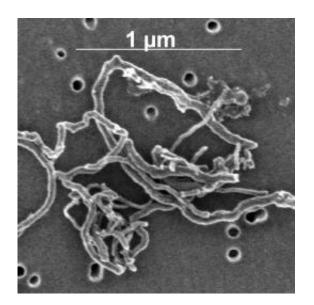
Atomic force microscope image of carbon nanotubes on a nuclear track filter membrane. Apart from the nanotubes, the 50 nanometer sized filter pores are clearly visible (image: E. Christalle).
