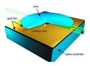
This image shows the design of a new type of invisibility cloak that is simpler than previous designs and works for all colors of the visible spectrum, making it possible to cloak larger objects than before and possibly leading to practical applications in "transformation optics." (Purdue University)
