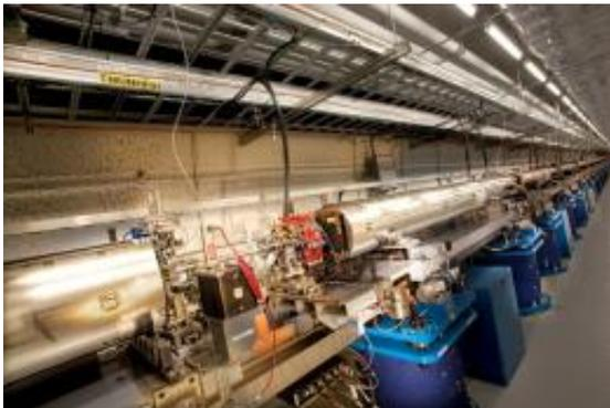
Only 12 out of a total 33 LCLS undulator magnets were needed to create the first pulses of laser light. Photo: Brad Plummer.
