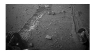
NASA's Mars Exploration Rover Spirit drove 6.98 meters (22.9 feet) southeastward on the 1,871st Martian day, or sol, of the rover's mission on Mars (April 8, 2009). As usual since losing the use of its right-front wheel in 2006, Spirit drove backward, dragging the immobile wheel. Image credit: NASA/JPL-Caltech.
