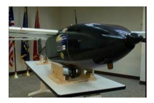
The Office of Naval Research's "Ion Tiger" UAV will test a hydrogen-powered fuel cell design, which can travel farther and carry heavier payloads than earlier battery-powered designs. Credit: The Office of Naval Research
