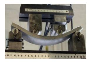
Self-healing concrete works because it can bend. When it's strained, many microcracks form instead of one large crack that causes it to fail. Here, a specimen is bending as a force of five percent tensile strain is being applied. Regular concrete would fail at .01 percent tensile strain.
