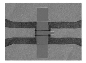
The gate of the transistor (the section in the middle) developed by Dr Moran is just 50 nanometres in length.
