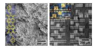
Scanning electron microscope images of (left) microwires synthesized using the researchers' method (inset is the chemical structure of the molecules); and (right) aligned microwires on a substrate (inset is the corresponding optical image). Credit: Oh et al. ©2009 PNAS.
