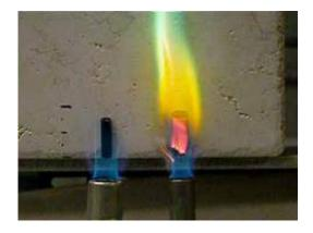
Pictured: two versions of the aerogel -- the RF-only version (left) and the mixed version (right).
