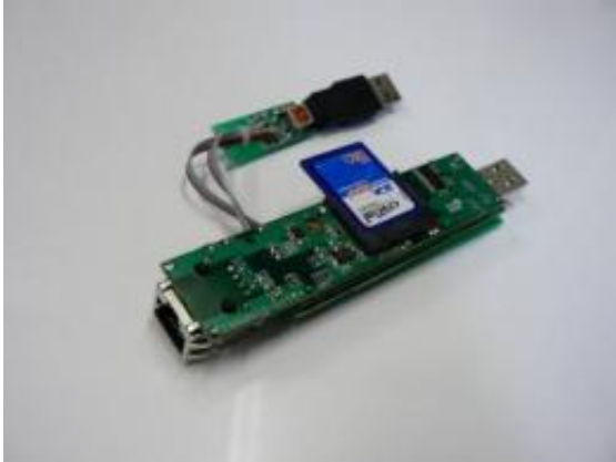
Figure 4 from the NSDI 2009 paper, "Somniloquy: Augmenting Network Interfaces to Reduce PC Energy Usage." The photograph captures the gumstix-based Somniloquy prototype -- Wired-1NIC version. Credit: Yuvraj Agarwal
