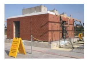
Engineers at UC San Diego will use data from seismic tests of this one-story reinforced concrete masonry structure to help make such structures more earthquake safe. Credit: UC San Diego
